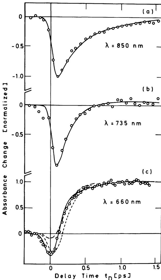
Figure 1. Time-dependent changes of absorption (negative values correspond to gain) induced by exciting femtosecond pulses at  $\lambda = 850$  nm (a),  $\lambda = 735$  nm (b),  $\lambda = 660$  nm (c). The solid curves are calculated using the decay kinetics discussed in the text. The broken curves are calculated for two different sets of amplitude parameters excluding the 50 fs kinetics.
