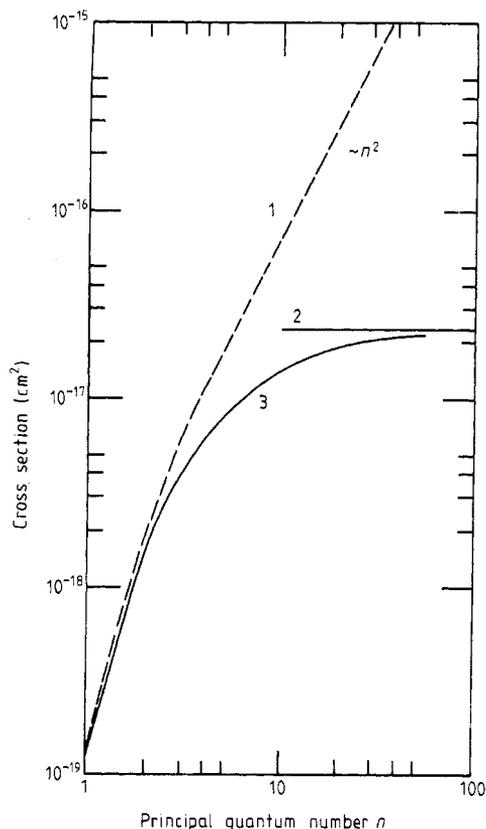
**Figure 2.** Calculated cross sections for electron loss from hydrogen-like sulphur ions in collisions with nitrogen atoms, as a function of principal quantum number  $n$ . Projectile energy is 125 MeV ( $v = 12.5$  au). 1, Born approximation without screening ( $Z_T^{\text{eff}} = 7$ ); 2, equation (3); 3, Born approximation with screening (see text).
