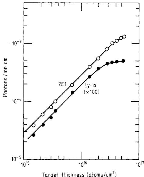
**Figure 1.** Absolute Ly- $\alpha$  and 2E1( $2s \rightarrow 1s$ ) intensities of sulphur ions, observed 10 cm behind a  $N_2$  gas target, as a function of target thickness. The Ly- $\alpha$  intensity shown signifies decay of long-lived Rydberg states.
