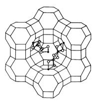
Chem-X space filling model for two (WO<sub>3</sub>)<sub>2</sub> dimers anchored to the 4Na<sup>+</sup> site II cations in the *a*-cage of Na<sub>56</sub>Y, (2c).
