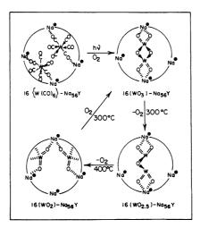
6. Summary of structures and anchoring schemes for a-cage encapsulated precursor 16{W(CO)<sub>6</sub>}-Na<sub>56</sub>Y as well as its photo-oxidation product 16(WO<sub>3</sub>)-Na<sub>56</sub>Y and corresponding reductive-elimination, oxidation-addition products 16(WO<sub>3-7</sub>)-Na<sub>56</sub>Y.
