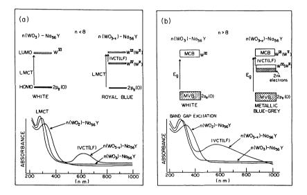
2. UV-visible reflectance spectra of  $n(WO_{3-x})$ -Na<sub>56</sub>Y for n < 8 and n > 8, where x = 0, 0.5, 1.
