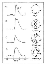
5. <sup>23</sup>Na MAS-NMR data for A) Na<sub>56</sub>Y B) 16(WO<sub>3</sub>)-Na<sub>56</sub>Y C) 16(WO<sub>2.5</sub>)-Na<sub>56</sub>Y and D) 16(WO<sub>2</sub>)-Na<sub>56</sub>Y
