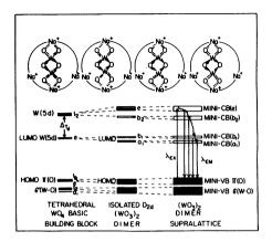
3. Evolution of a qualitative miniband electronic scheme for a (WO<sub>3</sub>)<sub>2</sub> dimer superalattice, 16(WO<sub>3</sub>)-Na<sub>56</sub>Y.
