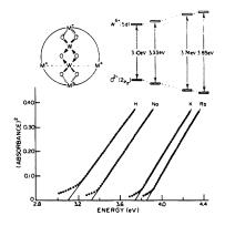
7. Experimental uv-visible absorption edges of a  $16(WO_3)-M_{56}Y$  supralattice, where M = H, Na, K, Rb together with the best computer fit to the absorption index of an allowed-direct band gap transition,  $a^{da} = K(E - E_g)^{V_2}$ . Inserts qualitatively illustrate the MVB/MCB energy levels for  $16(WO_3)-M_{56}Y$ .
