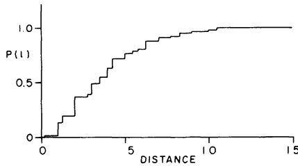
Fig.5 Diagram of a track pattern and the sum distribution of the distance between ionizations.
