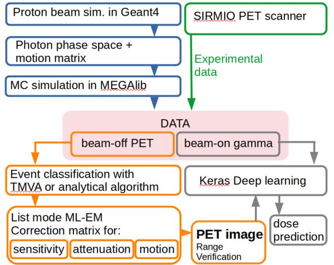
Figure 2: Framework architecture. Beam-on data are collected during the irradiation and beam-off data are collected in between the pauses of the irradiation (needed to accommodate the translation and rotation of the animal) or after it.
