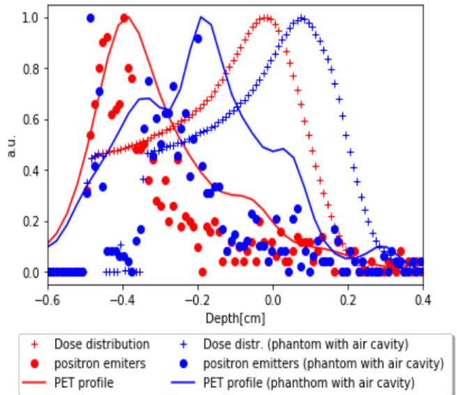
Figure 5: Orange and green lines are the PET image profile corresponding to the red and blue Bragg peak for energies separated by 0.5 MeV. The reference frame is set with the center of the scanner as central point.
