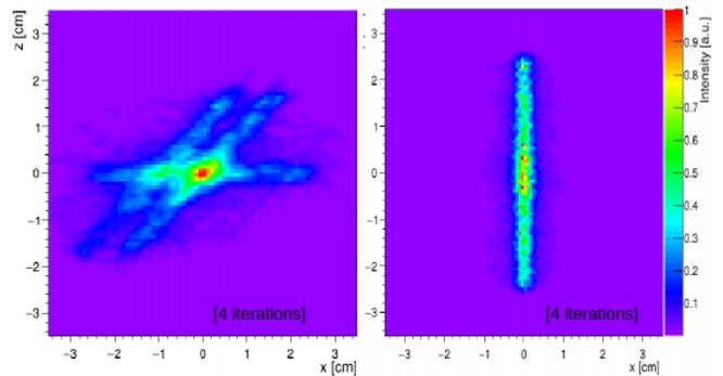
Figure 4: PET image and spatial distribution of  $\beta^+$  radioisotopes for a 50 MeV proton beam in a PMMA phantom.
