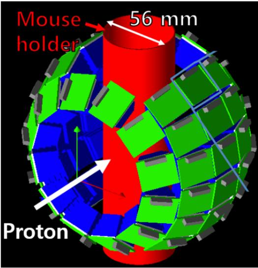
Figure 1: SIRMIO PET scanner design. The detector is composed of 56 scintillator blocks. The radius of the sphere is 72 mm. The mouse holder can be moved to place the tumor in the center of the scanner field of view.
