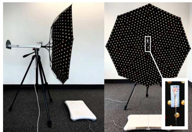
**Fig. 1** Experimental setup consisting of a height-adjustable inverted umbrella forming a dome around the horizontal axis for visual stimulation in the roll plane, a subjective visual vertical system with a pointer on the rear side, a piece of cardboard on a metallic rod depicting a giraffe in the center of the dome (see insert) and a posturographic platform (bottom)
