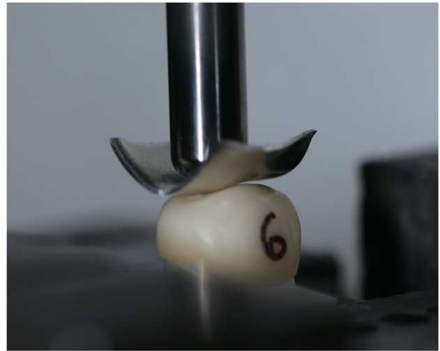
Fig. 3 A Zolid RS/HS specimen (1.0 mm, initial) mounted for the fracture load test
