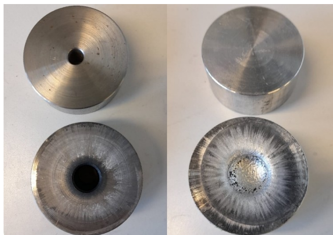
Figure 8. Steel block (left) and aluminum block (right) before (top) and after (bottom) the detonation of 1300 mg PETN.
