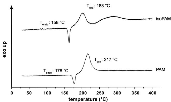
**Figure 9.** DTA measurement of iso-picramic (2, top) acid and picramic acid (bottom) [12].
