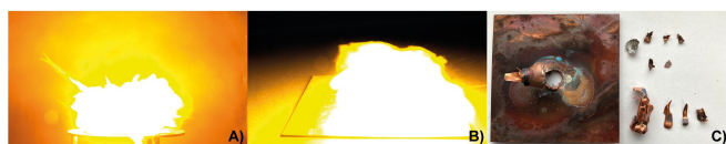
Figure 11. A) Deflagration of 9 during hot plate test; B) Deflagration of 9 during hot needle test; C) Positive PETN initiation test with 50 mg of 9.
