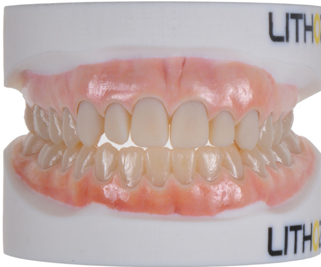
FIGURE 4 Colored model produced using the Stratasys PolyJet method in multimaterial 3D printing.
