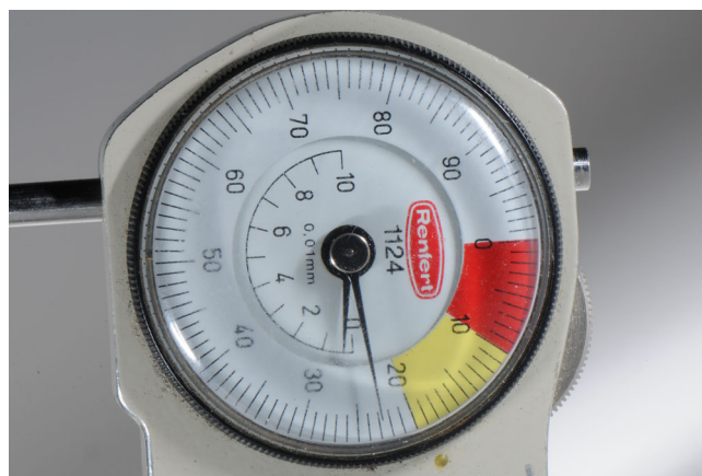
FIGURE 12 The total layer thickness of the veneers was 0.225 mm (0.2 mm veneer and 0.025 of glazing material).
