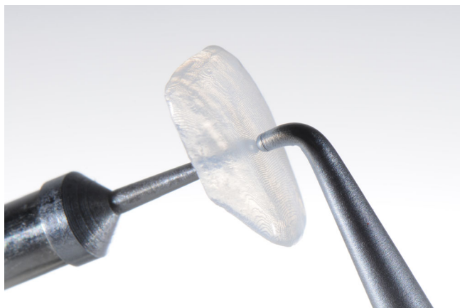
FIGURE 11 The layer thickness of the ultra-thin veneers was checked with a precision measuring instrument after glaze firing.
