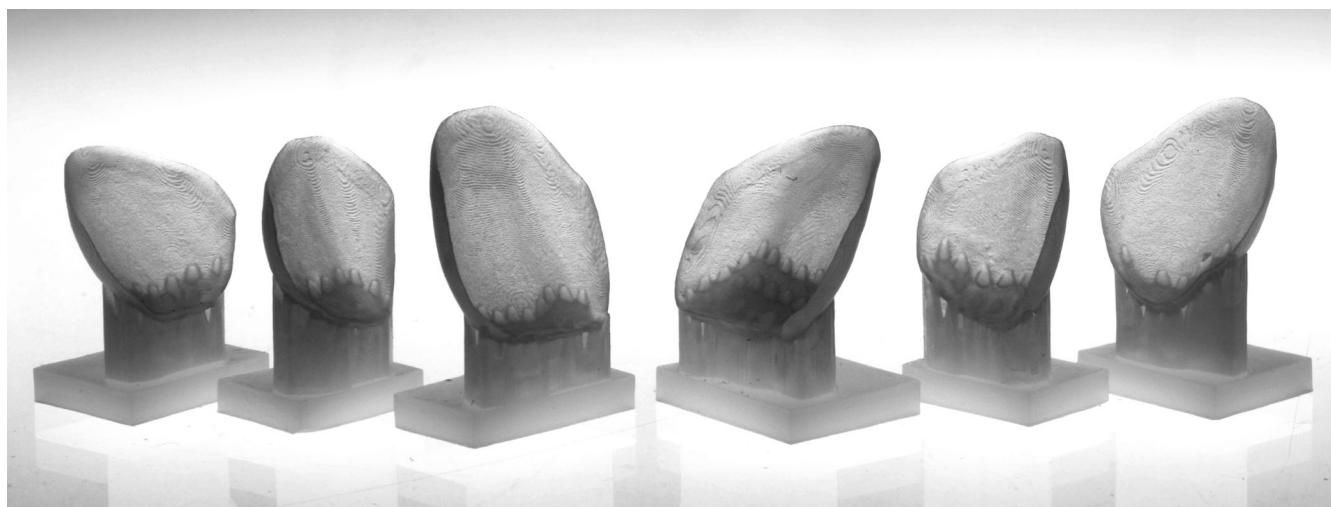
FIGURE 7 Veneers after thermal treatment (debinding, sintering, and crystallization).
