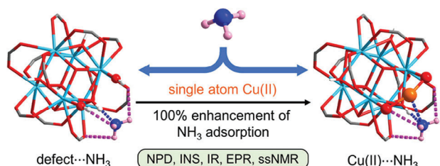
Figure 36. Ammonia adsorption in UiO-66 and defective UiO-66. Defective UiO-66 metal-organic frameworks show enhanced \text{NH}_3 uptake and dynamics. Reproduced with permission. [160] Copyright 2022 American Chemical Society.
