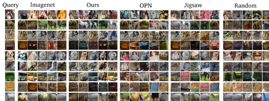
Fig. 3. Unsupervised evaluation of the feature representation by nearest neighbor search on the VOC07 dataset. For every test sample we show the Top5 nearest neighbors from the training set (Top1 to Top5 from left to right) using the cosine distance of the pool5 features. We compare the models from (i) supervised training with the Imagenet classification task, (ii) our spatiotemporal approach, (iii) OPN as a temporal approach [28], (iv) Jigsaw as a spatial method [34] and (v) a random initialization.
