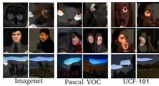
Fig. I.1. Rows: Top activations of 3 different conv5 neurons across three datasets (columns). Note, that the neurons exhibit the same behavior in all datasets; The first unit focuses on eyes, the second on faces and the third on sky in a landscape.
