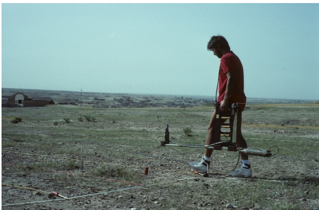
Fig. C2.1: Magnetometer prospecting in Assur in April 1989, with Jörg Fassbinder operating the handheld caesium magnetometer (Varian 101) in the so-called “variometer” configuration. Photo by Manfred Stephani.
