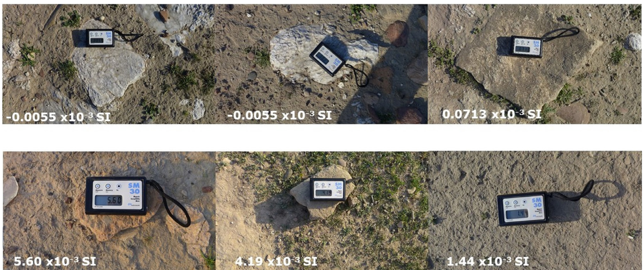
Fig. C2.5: Magnetic volume susceptibility measurements taken in situ in Assur with a handheld Kappa-meter SM30 (Zh-Instruments). Clockwise from top left: Gypsum rocks (diamagnetic, with “negative” kappa value), limestone, baked bricks and topsoil.
