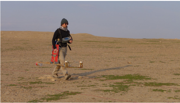
Fig. C2.3: Magnetometer prospecting in Assur in February 2023, with Jean-Jacques Herr operating the handheld duo-sensor caesium magnetometer. Photo by Jörg Fassbinder.
