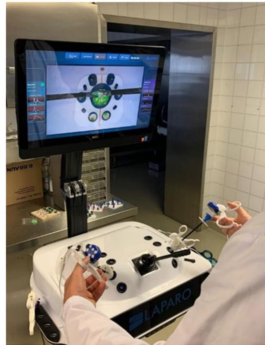
**Fig. 2** Test setup of laparoscopy trainer. The inertial sensors are attached to the instruments
