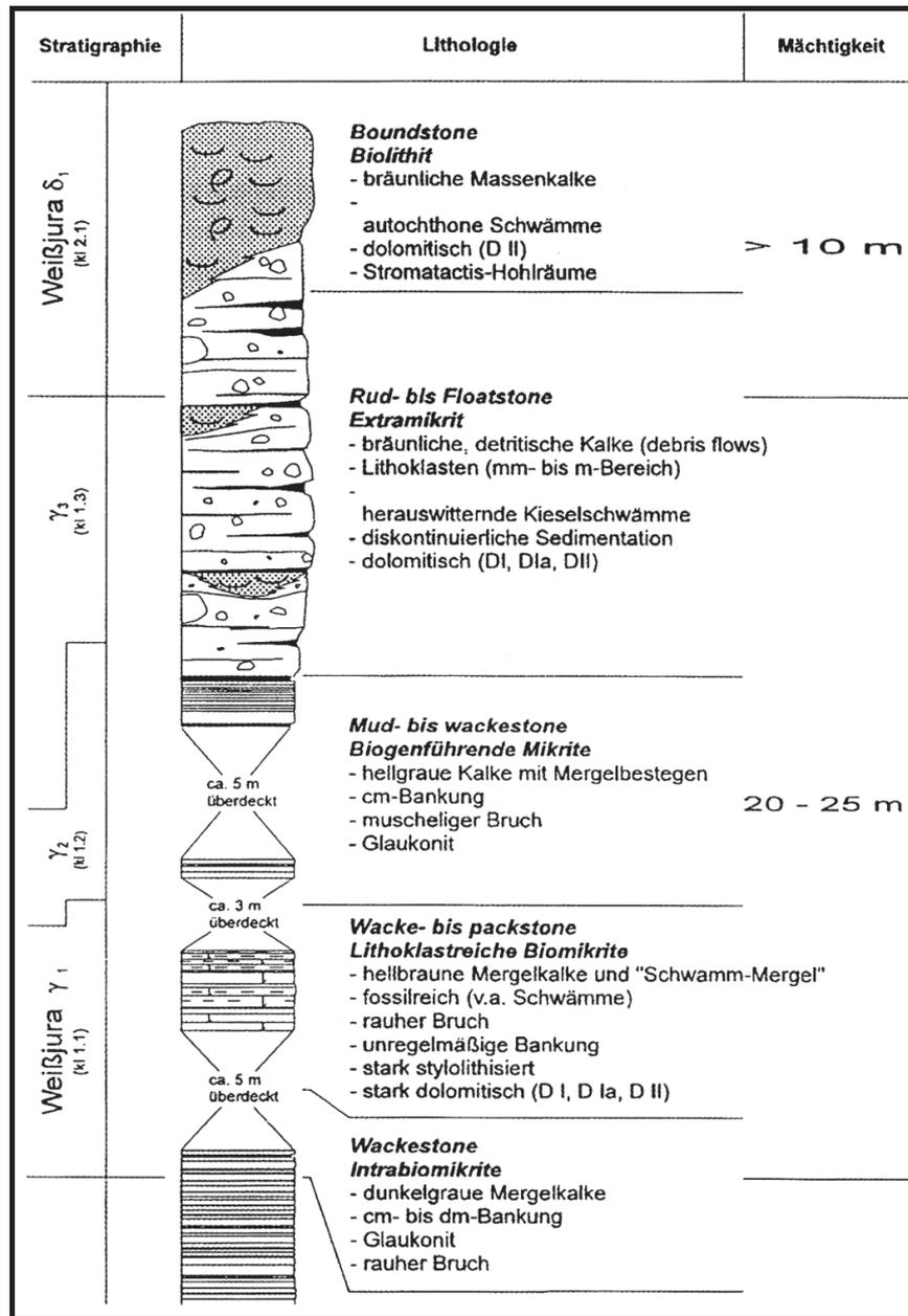
**Figure 9:** The profile up to the Schießfels near Hardt which marks the beginning of the growth of sponge-algal buildups in the uppermost Malm gamma (from TARASCONI 1996).
