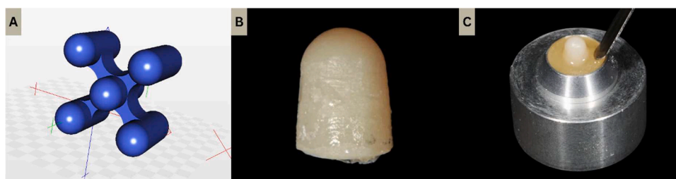
Fig. 3. A. Master ceramic antagonist STL file. B. milled and separated ceramic antagonist. C. embedded ceramic antagonist. D. milled master abutment.
