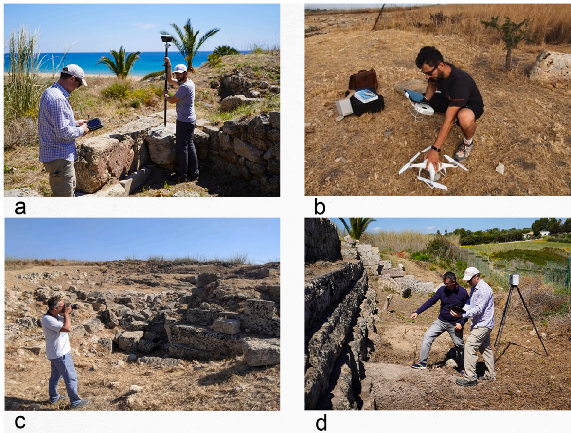
Fig. 8. a) HADES project team members are seen collecting GNSS survey points inside Tower 3; b) a team member is seen setting up a drone to gather low altitude aerial photographs of the agora district for 3D mapping purposes; c) a Team member is seen capturing photos of North Gate’s Tower A for 3D mapping purposes; d) Team members are seen reviewing Terrestrial LiDAR data of the Northeast Wall in the field using a tablet. Photographs a-c) by Davide Tanasi, photograph d) by Dario Calderone.
