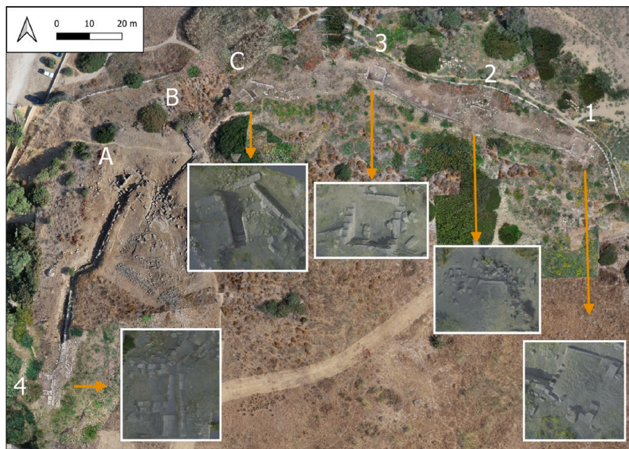
Fig. 13. Orthophoto of Heloros' fortifications derived from drone-based photogrammetry data showing the location and details of Towers A, B, C, and 1, 2, 3, 4 (the towers are visualized as renders from terrestrial Lidar point clouds). Orthophoto and 3D models by Dario Calderone.
