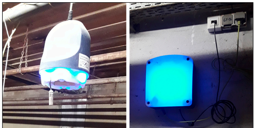
Figure 1. Left picture: SoundTalks ® monitor in science mode (blue led). Right picture: Plugged gateway in science mode (blue led).
