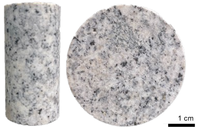
Figure 1. Photographs of a representative core for porosity measurements and uniaxial compressive strength testing, and a disc for Brazilian tensile strength testing. Phenocrysts of feldspar (pale pink), with finer grains of quartz and plagioclase (both white to pale grey) and clusters of mica (dark grey to black) are visible.
