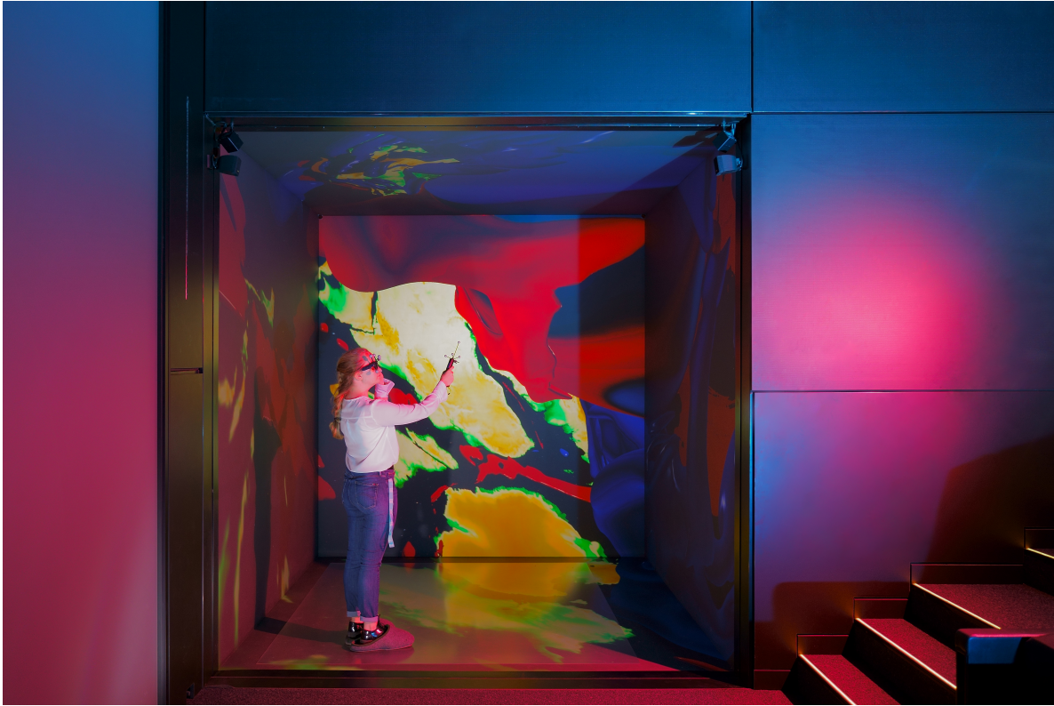
Figure 2: A user in the CAVE interacting with the visualization of convection streams within the Earth's mantle for a project of geophysics.
