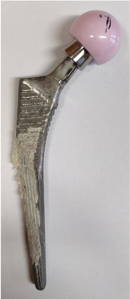
Fig. 1. Explanted example of the universal head-neck adapter with a lateralized configuration, a ceramic head, and an uncemented stem, with signs of mechanic wear and tear due to revision surgery.
