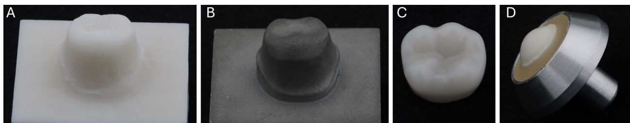
Fig. 2 Specimen preparation; A : polymer abutment with dentin like E-modulus, B : CoCrMo abutment, C : feldspar ceramic crown (FEL), D : steatite antagonist for mastication simulation
