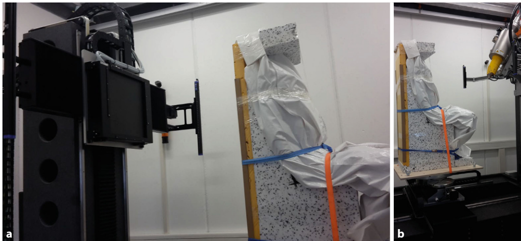
Fig. 1 ◀ a, b Corpse in a sitting position on the constructed styrofoam seat in front of the X-ray source on a rotating table ( b ) and with the flat panel unit behind ( a )
