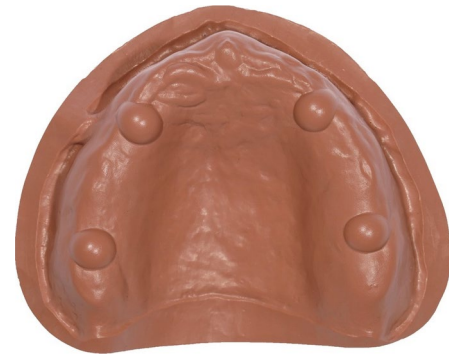
Fig. 1 Testing model milled from PEEK
