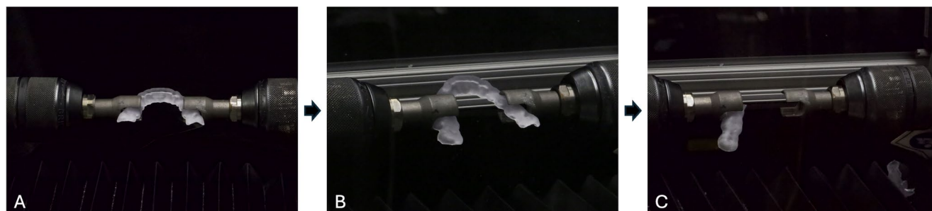
Fig. 6 Testing device. A, Occlusal device clamped in testing device. B, Occlusal device rotating during the test. C, Fractured Occlusal device—end of the test
