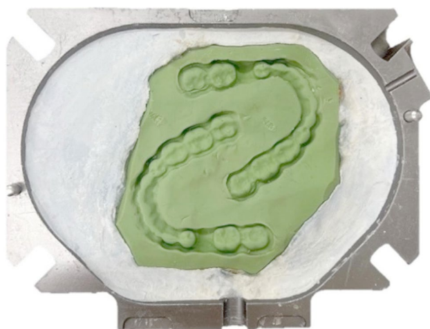
Fig. 5 Injection technique. Occlusal device geometry embedded in a flask
