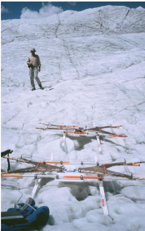
Photo 4: Ground penetrating radar antennas.
