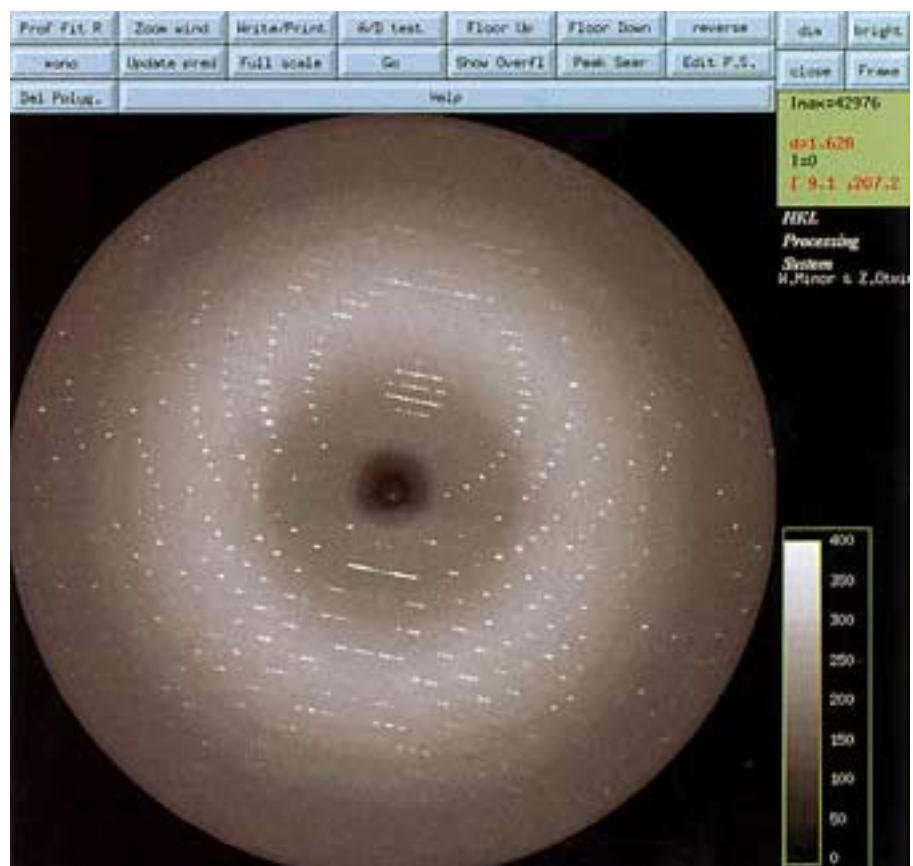
Fig. 9. A 1° oscillation photograph of CG-16 collected on a Rigaku RU200 rotating anode generator operating at 5.4 kW. The diffraction pattern in this film extends to 2.1 Å resolution.
