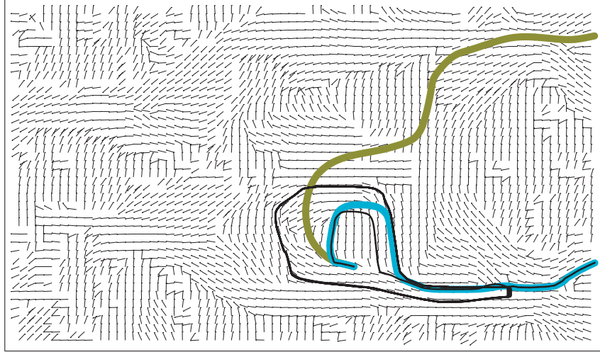
Figure 2: Examples of tracks generated by Algorithm T2 with different values of "braking" parameter c_1 : c_1 = 1 (dark wide line), c_1 = 3 (light wide line), c_1 = 5 (narrow black line). The values of other parameters: \Delta t = 0.1 , c_0 = 1 , \sigma = 0 . The vector field and the starting point for tracking are the same as for Figure 1.
