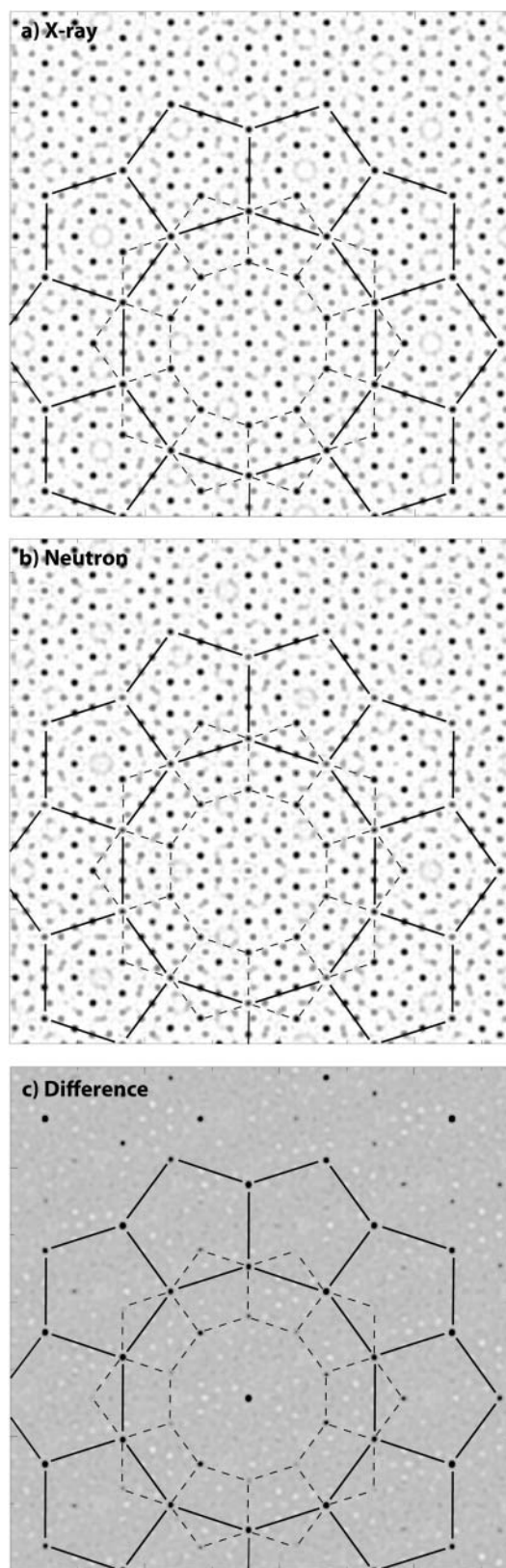
Fig. 3. 75 \text{ \AA} \times 75 \text{ \AA} sized X-ray, neutron and difference scattering density maps as obtained by LDE. The Co atom positions are clearly identified in the difference map (dark difference densities have a higher density in the X-ray than in the neutron case, the gray background indicates the zero level). As indicated, Co atoms arrange in pentagonal units, which form decagonal rings. Dashed and solid line motifs are related by a scale factor \tau .
