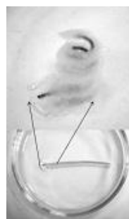
[Figure 2: Hydrogel-based self-bending of the shaft]
