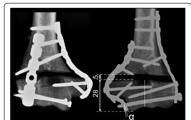
Figure 1 Anteroposterior radiographs of an operated bone pair. Left: LCP construct with 90° plate arrangement. Right: "Frame" technique with interconnection between both plates parallel to the joint surface for establishment of a "U"-shape configuration. The interconnection screw engages with the reconstruction plate. \alpha indicates an oblique orientation of the plate, which further promotes the anchorage of the screw. Numbers are given in mm.
