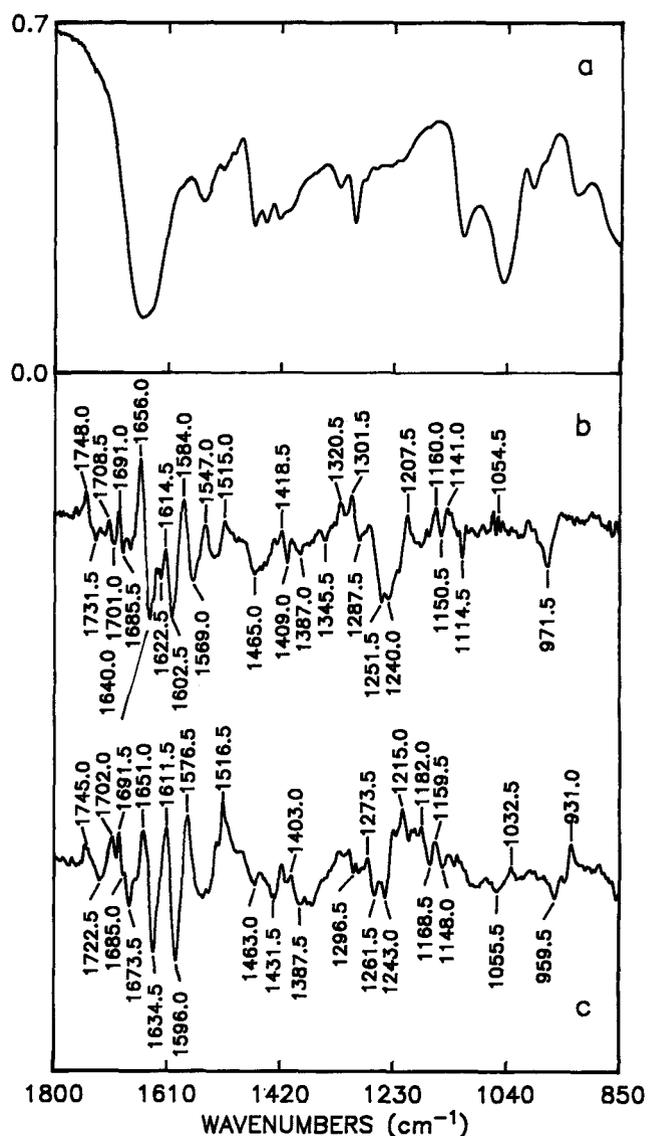
Fig. 6. Infrared spectra of phytochrome. (a) Single-beam spectrum of a hydrated film sample of phytochrome with intensity on the ordinate. (b, c)  $P_r - P_{fr}$  infrared difference spectra of a hydrated film sample of phytochrome hydrated with  $^1H_2O$  (a) and  $^2H_2O$  (b) with absorbance on the ordinate. Each difference spectrum represents the sum of 20 individual difference spectra obtained from 10 illumination cycles as described in Materials and Methods
