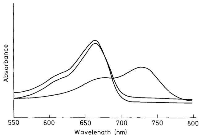
Fig. 5. Visible absorption spectra of the hydrated film samples of phytochrome to demonstrate the good photoreversibility. The lower trace of the phytochrome spectrum was obtained by illuminating the  $P_r$ - $P_r$  mixture with far-red light
