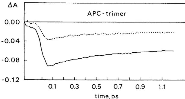
Figure 2. Absorption recovery of APC trimers at 615 nm (Sample No 2) with probe pulse polarization parallel (solid line) and perpendicular (dashed line) to the exciting pulse.
