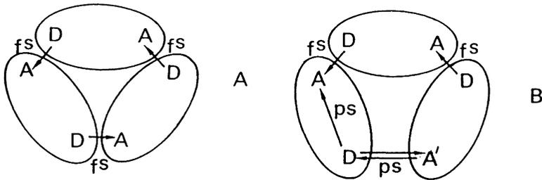
Figure 5. A model for fast energy transfer pathways in intact trimers (A) and in partly disintegrated trimers (B).
