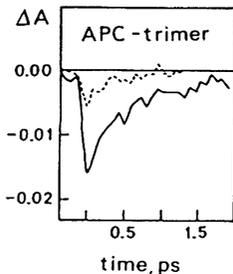
Figure 1. Absorption recovery of allophycocyanin trimers at 615 nm (Sample No 1) measured with probe pulse polarization parallel (solid line) and perpendicular (dashed line) to the exciting pulse.
