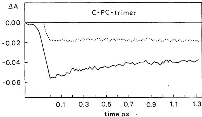
Figure 3. Absorption recovery of C-phycoerythrin trimers at 615 nm with probe pulse polarization parallel (solid line) and perpendicular (dashed line) to the exciting pulse.
