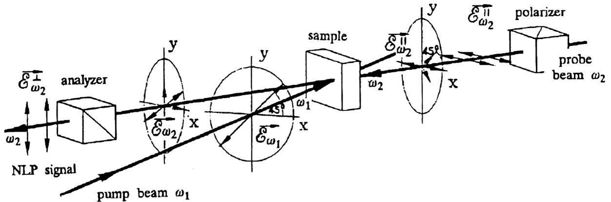
Fig. 1. The principle of nonlinear polarization spectroscopy in the frequency domain. The probe wave is linearly polarized at  $45^\circ$  to the linearly polarized pump beam. The pump beam induces dichroism and birefringence in the sample. The dichroism and birefringence lead to a component orthogonal to the initial probe polarization. This orthogonal component of the probe wave is the signal of the nonlinear polarization spectroscopy
