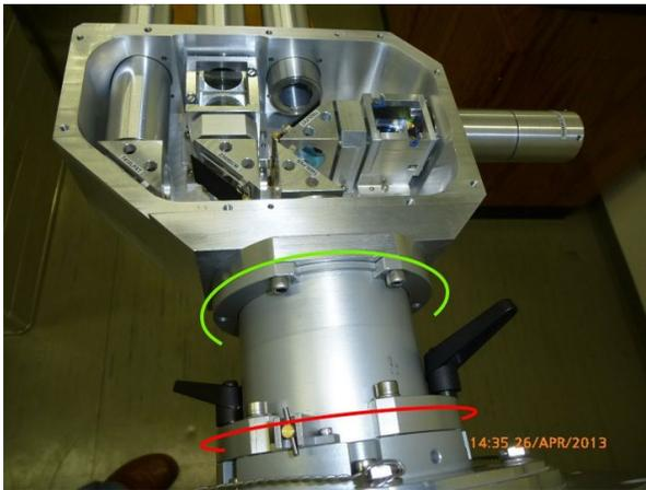
**Figure 2** Inside of the receiving optics module of POLIS-6 with the top cover removed. The telescope mount is at the image bottom, indicated by the red circle, which also provides the rotation with the fixed  $\pm 45^\circ$  and  $0^\circ$  positions of the module with respect to the laser/telescope assembly (see Fig.1). The green circle indicates the rotation mount for exact  $0^\circ$  adjustment. At the right and top the detector modules are protruding.
