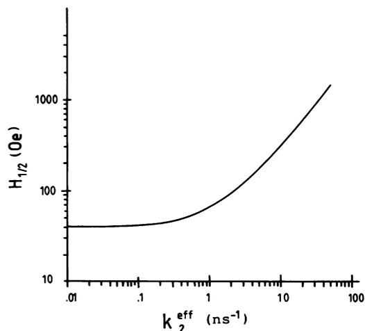
FIGURE 4 Dependence of the half-width of the magnetic field effect on the spin dephasing rate  $k_2^{\text{eff}}$  for a probing time of 7 ns, one effective nucleus,  $k_S^{\text{eff}} = 0.039 \text{ ns}^{-1}$ ,  $k_T^{\text{eff}} = 0.74 \text{ ns}^{-1}$  and  $J^{\text{eff}} = 3 \text{ Oe}$ .
