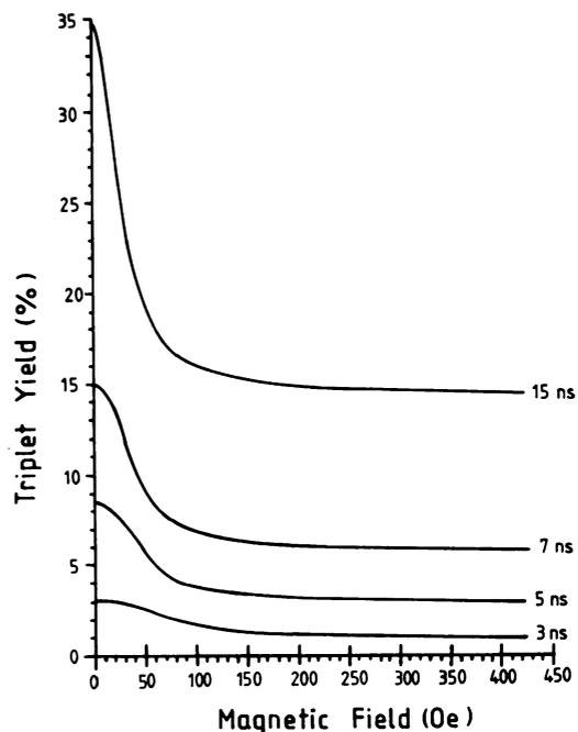
FIGURE 3 Magnetic field dependence of the triplet yield at different times calculated for one effective nucleus by least-square fitting of quantities derived from Fig. 2:  $\phi_T(0)$ ,  $\phi_T(0)/\phi_T(\infty)$  and the half-width of the magnetic field effect.
