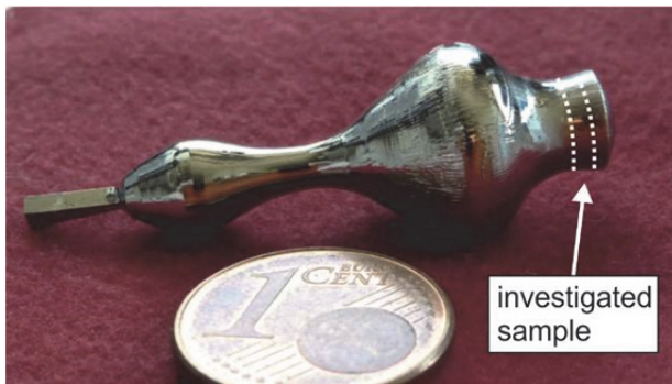
Figure 3. \text{Pd}_2\text{Ga} solid-solution single crystal grown by the Czochralski method from Ga-rich solution. The marked section represents the investigated slice of the crystal.
