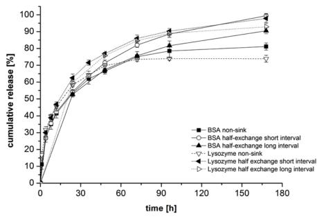
Fig 7. Cumulative release of BSA or lysozyme from alginate hybrid gels. Investigations were carried out using non-sink conditions, half-exchange within short intervals or half-exchange within long sampling intervals ( $n = 3 \pm SD$ ).
