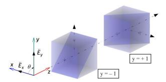
**Figure 3.** Definition of the global coordinate reference system and the binary operator y with respect to the incident plane of the polarising beam splitter. If the polarising beam splitter orientation parameter y = +1, the vibration of the horizontal linear polarisation with vector  $E_x$  is parallel to the plane of incidence, while for y = -1 it is perpendicular.
