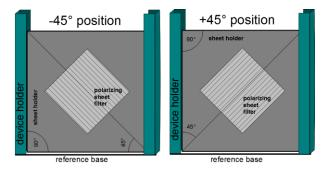
Figure 5. Simple holder for sheet filters (linear polariser or  $\lambda/4$  plate) with accurate positioning for the  $\Delta 90$  calibration.
