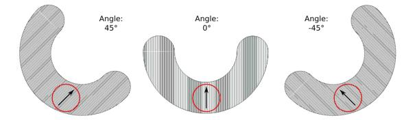
**Figure 6.** Linearly polarising sheet filter cut-out for use in a rotation mount. The optical axis of the filtered light beam is in the centre of the red circle. Reproduced with permission from Kölbl (2010).
