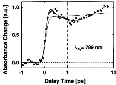
Fig. 3. Transient absorption (points) measured at a probing wavelength of 789 nm. The broken curve was calculated with a time constant of 4.5 ps while two time constants of 0.6 ps and 4.5 ps are used for the solid model function. The data show that the fast time constant is required in order to simulate the data points.
