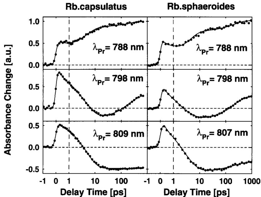
Fig. 4. Comparison of the transient absorption data of isolated RC of *Rb. sphaeroides* (right) and RC in whole membranes of *Rb. capsulatus* (left part). The probing wavelengths were taken in the  $Q_y$  absorption band of the monomeric bacteriochlorophylls. One observes a good qualitative agreement between the two types of reaction centers in this very complex spectral range.
