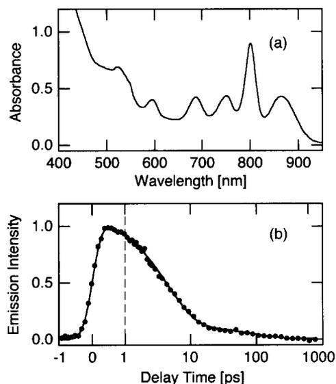
Fig. 1. (a) Absorption spectrum of the reaction centers of *Rb. capsulatus* strain U43 (pTXA 6–10) used in the time-resolved experiments. (b) Transient emission data from the RC after excitation at 865 nm. The data points are modelled by a biexponential model function (solid line) with time constants of 4.5 ps and 90 ps.
