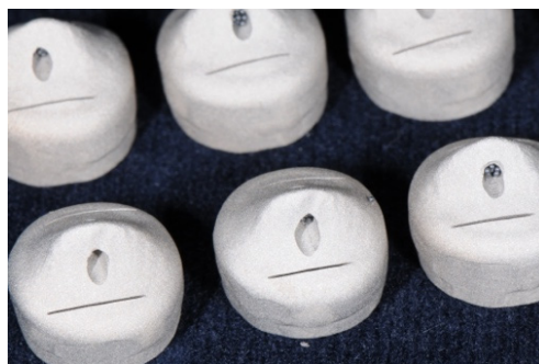
Figure 3. Cobalt-chromium secondary crowns with a hole for the pull-off test directly after sintering.
