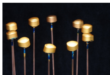
Figure 5. Primary crowns with gold copings on rods after the electroforming process.
