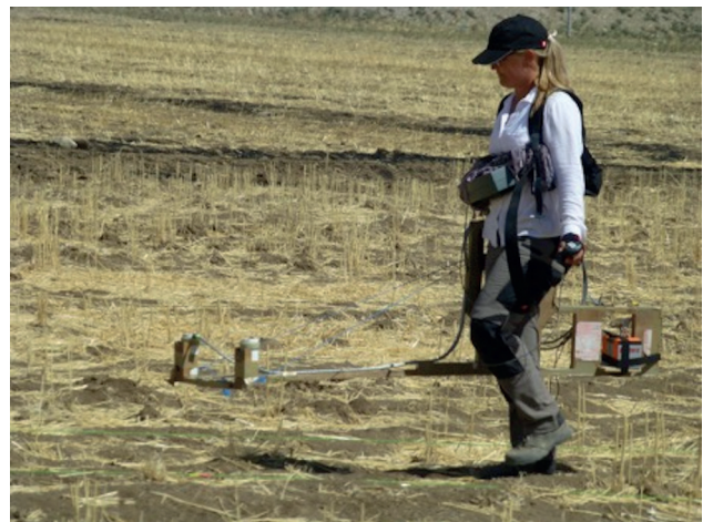
Fig. B1b: Magnetometer prospection with the handheld total field magnetometer Geometrics G-858 in duo-sensor configuration. Photo by Jörg Fassbinder.
