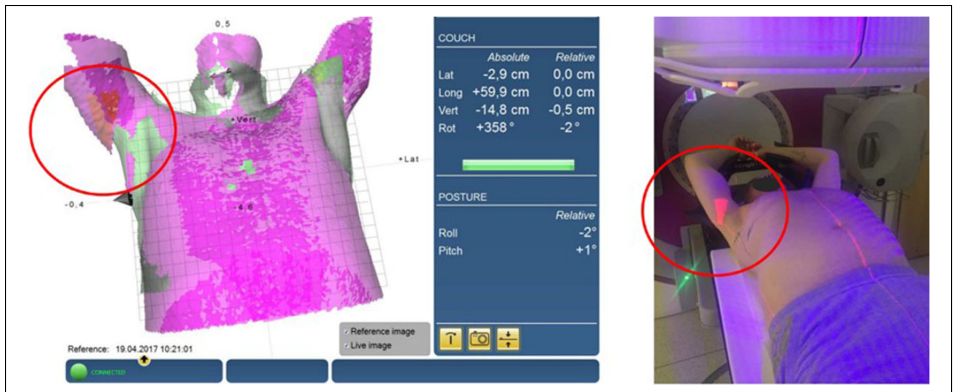
Figure 2. Positional deviations projected onto the patients' surface (screenshot of Catalyst software c4D [C-Rad AB]). Local deviations outside the tolerance limits compared to the reference scan are marked in red.
