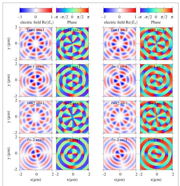
**Figure 3.** Electric field component  $Re(E_x)$  and phase of the scattered electric field of an Archimedean spiral with m=4 elements for OAM light excitation with  $\ell=\pm 1, \pm 2$  and  $s=\pm 1$ .
