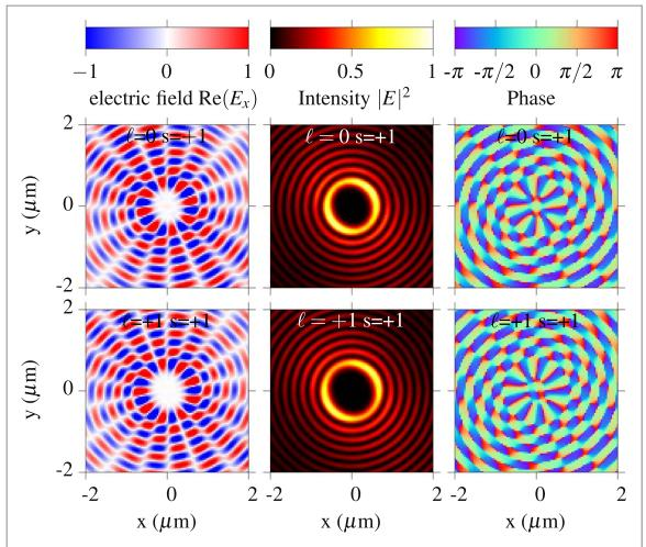
**Figure 4.** Electric field component  $Re(E_x)$ , intensity and phase of the scattered electric field of an Archimedean spiral with m=4 elements for an excitation with OAM values of  $\ell=0,+1$  and circular polarization s=+1 at the wavelength  $\lambda=d/2=400$  nm.
