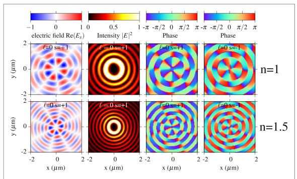
**Figure 2.** Electric field component  $Re(E_x)$ , intensity and phase of the scattered electric field of an Archimedean spiral with m=4 elements for plane wave excitation with varying polarization  $s=\pm 1$ . The refractive index of the embedding medium is n=1 (top row) and n=1.5 nm (bottom row).
