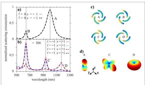
**Figure 5.** Scattering cross-section of Archimedean spiral with radius  $r_0 = 100$  nm for (a) non OAM light with  $\ell = 0$  and for (b) OAM light with  $\ell = \pm 1$ . The corresponding (c) surface charge distribution (yellow = positive charge and blue = negative charge) and (d) directional radiation pattern at resonance wavelength for different resonances (red = high R and blue = low R).
