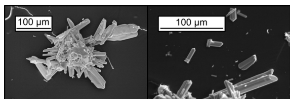
Figure 1. SEM images of \text{Ca}_2\text{PN}_3 . Rod-shaped single-crystals > 100 \mu\text{m} are observed.
