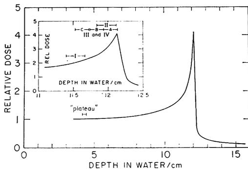
FIG. 1. Depth-dose distribution for a beam of 3.9 GeV nitrogen ions; showing the position at which seedlings were irradiated in the various experiments.
