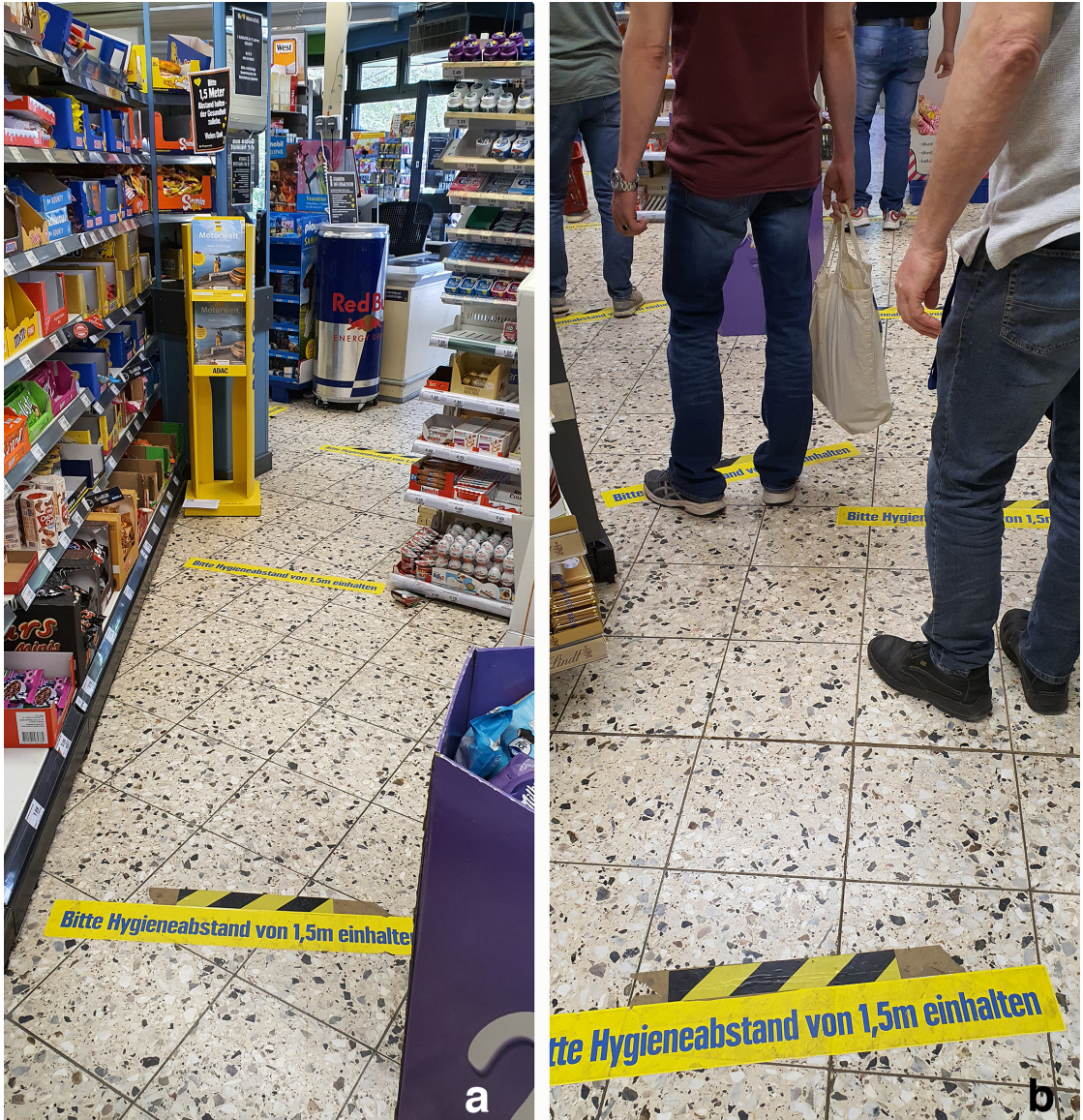
Figure 1. (a) Labels on the floor of a convenience store mandating a distance of 1.5 m. The yellow labels are spaced 1.5 m apart in one direction only. (b) People queuing and violating distance requirements because only frontal distances have been considered in the design of the labels.
