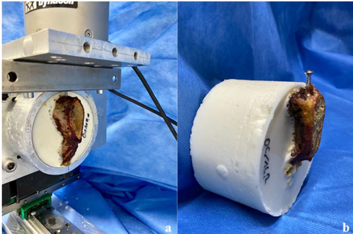
Fig. 1 Specimen embedded and mounted on the Instron testing machine during testing (a) and after screw pull-out (b)
