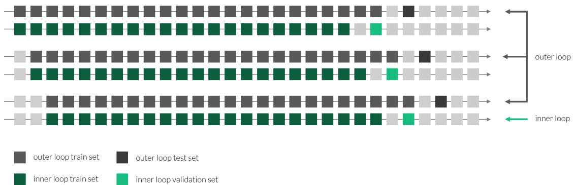
Figure 4.2: Illustration of the nested time series walk-forward validation. Example, based on prediction horizon of 2 steps.
